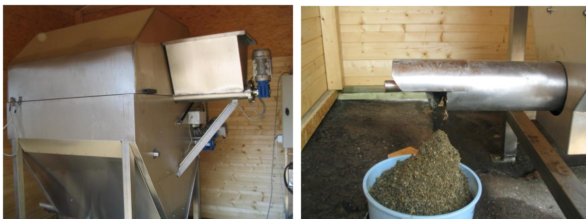
Fig. 4 Device for mechanical grinding of plants substrates - photo
