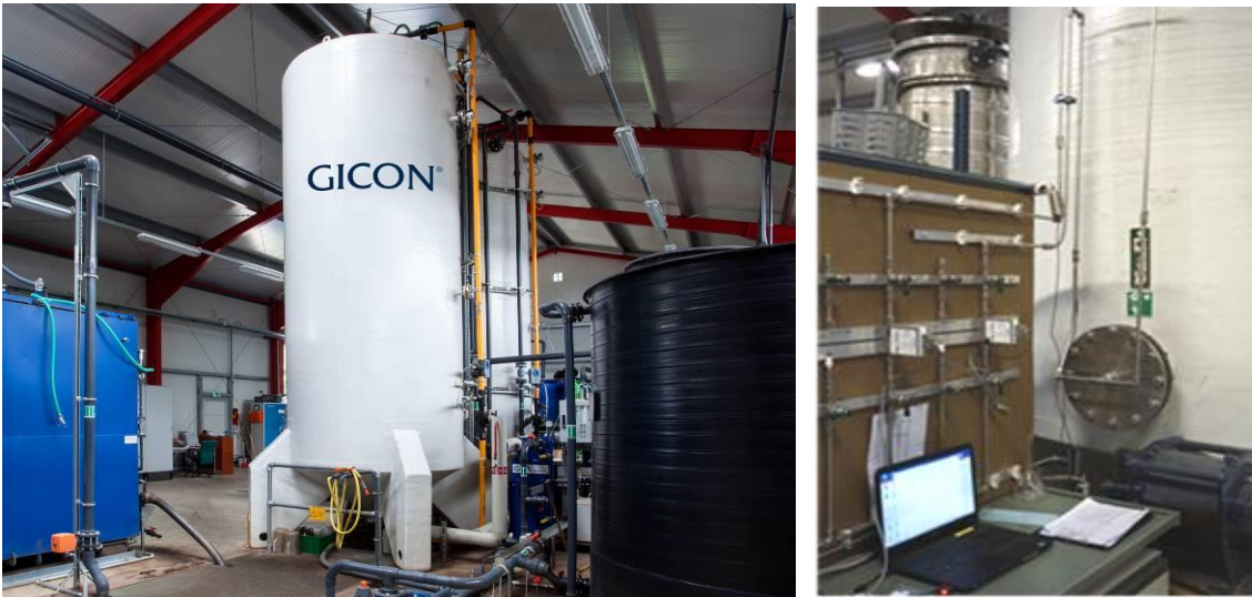
GICON-Technikum – large scale trickle-bed reactor for methanation
